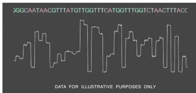
Fig. 4: The squiggle is the trace of the signal measured by the MinION. For the illustration, a sequence after basecalling was added above, for a visualization of a real signal see figure 11
